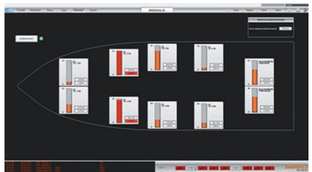
Figure 3: Add on for Norwegian Institute: tank level measurement
